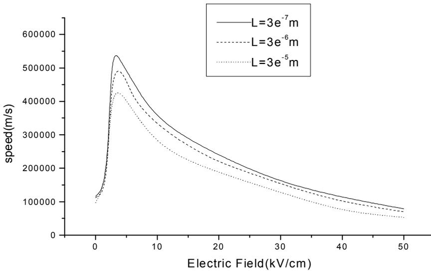
**Figure 8 :** *Speed profile according to the field E in InAs for various lengths of material*
