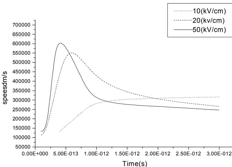
**Figure 5 :** *Evolution of speed versus time for various fields E*
