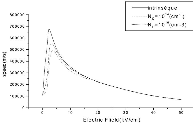
**Figure 6 :** *Speed profile according to the field E in InAs for different doping*
