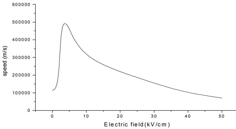
**Figure 1 :** *Speed profile according to the electric field E in InAs*
