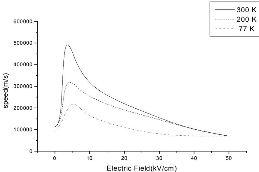
**Figure 7 :** *Speed profile according to the field E in InAs for different temperatures.*
