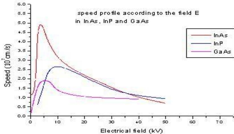
**Figure 3 :** Speed profile  $\varepsilon$  according to the field  $E$  in InAs, InP and GaAs
