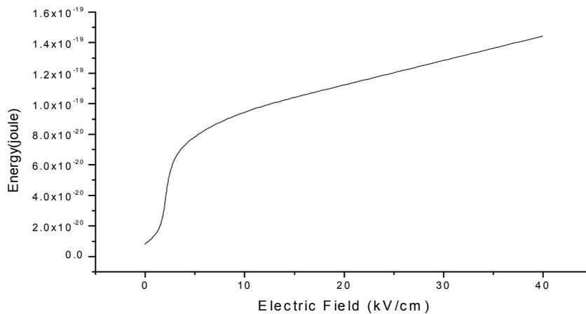
**Figure 2 :** *Evolution of energy over electric field E in InAs*
